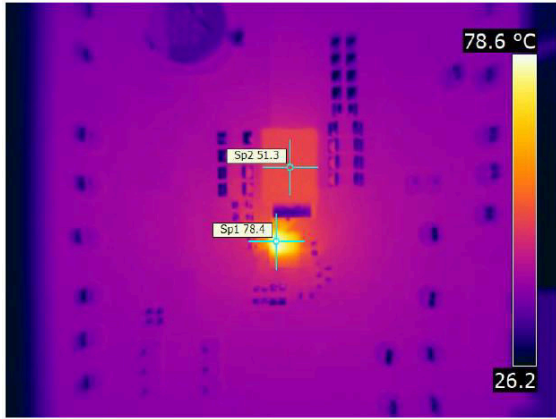
图 6-13. Thermal Image at 15-A Output Current
